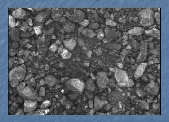
Images are acquired by cameras placed above dump trucks or conveyor belts
