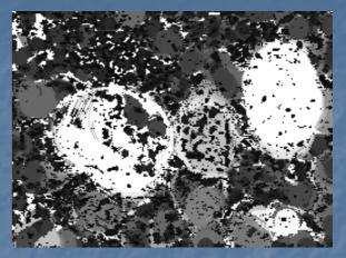
Various factors (fine particles, textured zones, crystalline materials, etc.) produce very noisy ultimate openings and granulometric functions
