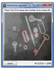
Interactive segmentation display (left), result of the segmentation after the definition of 4 markers, one in each segmented object and one in the background (right).
