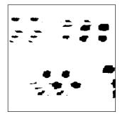
Initial particle2 image (left). Opening by an horizontal doublet of points at distance 30 (middle) and at distance 45 (right).
