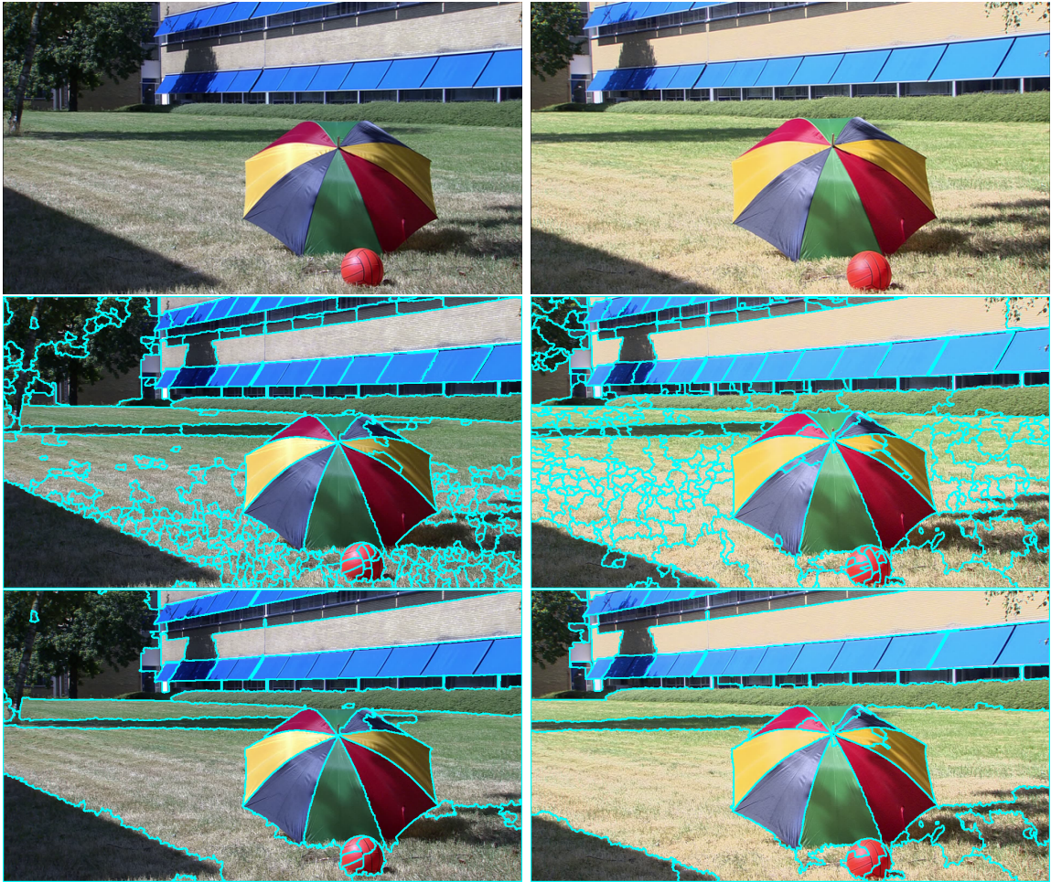
Figure 2: Region segmentation and fusion. Row 1: reference (left) and input (right) images. Row 2: watershed segmentation. Row 3: region fusion. The watershed line is one-pixel large, but we increase their thickness for better visualisation.
