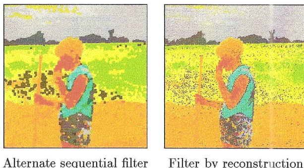
Fig. 4. Morphological filters applied on the reduced color image.
