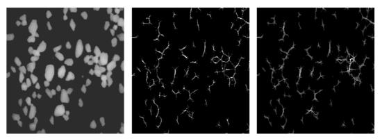
Initial image Ultimate erosion Associated function Figure 3: Greytone ultimate erosion for a greytone image
