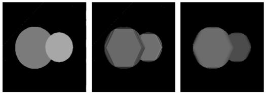
Initial image Ultimate opening Granulometric function Figure 5: Ultimate opening and granulometric function
