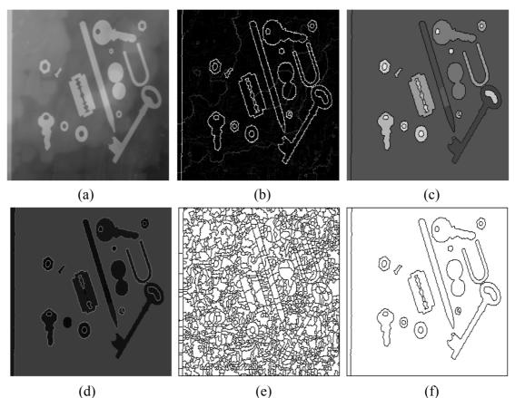
*Figure 17*: Initial image (a), valued watershed of gradient (b), supremum of pilings  $\theta$  (c) Associated function q (d), initial contours (e), preserved contours after piling process (f) 7. Conclusions
