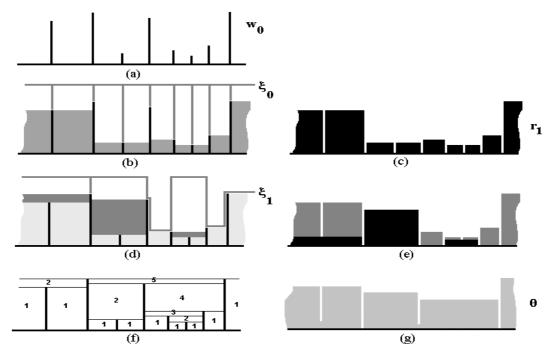
Figure 16: Hierarchical segmentation from residues of pilings (a) Initial watershed, (b) construction of  $\psi_1$ , (c) first residues, (d) construction of  $\psi_2$  (in grey) and residues  $r_2$  (dark grey), (e) supremum of  $r_1$  and  $r_2$ , (f) the various piles and their order of appearance, (g) final  $\theta$  function (supremum of all residues)
