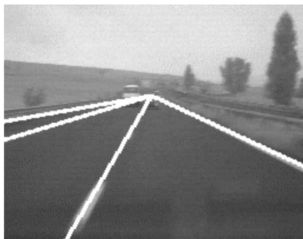
Figure 3 - Segmentation in tracking mode, using a road model (rear view).
