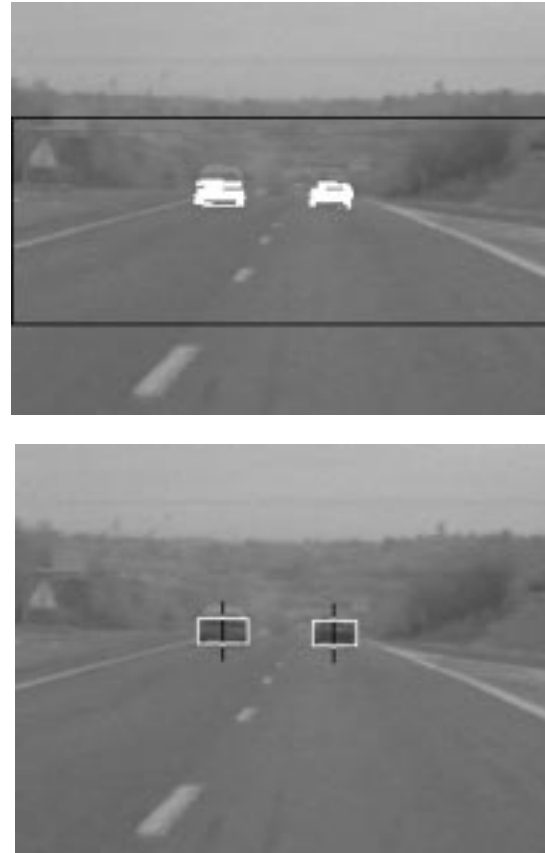
Figure 6: Detection of the dark zone in front of vehicles (up) and corresponding bounding boxes (down)
