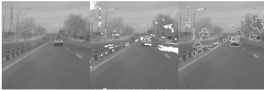
Figure 5. The significant minima in an image are used as markers in the gradient watershed image.
