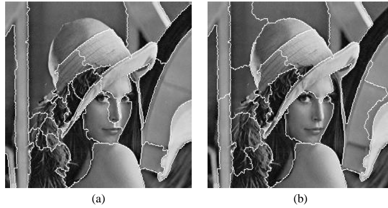
Figure 6. Comparison between different hierarchies. (a) Contrast-based Waterfall, 36 regions. (b) Volume based Waterfall, 24 regions.
