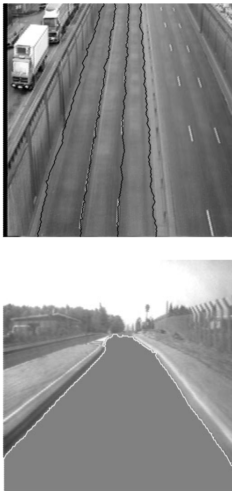
Figure 16. Examples of watershed segmentation of traffic pictures Lanes segmentation (upper), road segmentation (lower)
