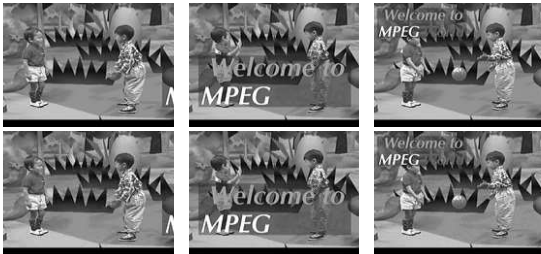
Fig. 13. Coding results for the Children sequence coded at 320 Kbits/s and 15 frames/s. First row: original frames 6, 100, 192. Second row: coded frames
