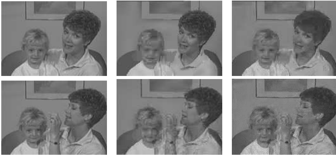
Fig. 15. Comparison between selective and non-selective coding of the head of the mother in frames number 0 (first row), 84 (second row) of the Mother and Daughter sequence. Left: original frames, Center: selective coding, Right: non-selective coding.
