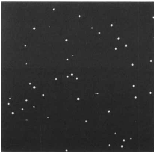
Fig. 15. Spheres in Fig. 14 selected and isolated from the fibres with the top hat filter.
