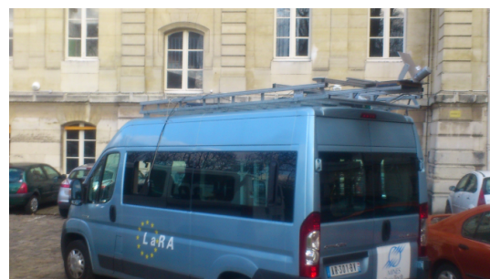
Figure 3: MLS system L3D2 from CAOR-MINES ParisTech
