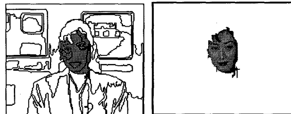
Figure 4 - Example of face detection for sequence Akiyo .
