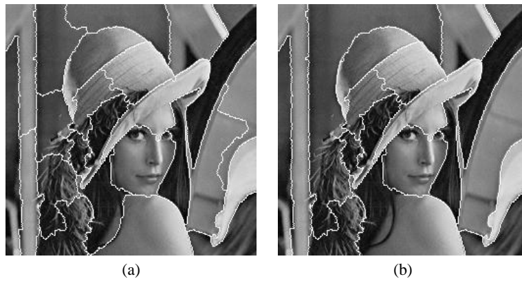
Figure 7. Elimination of low contrasted frontiers. (a) volume based waterfall (24 regions). (b) From (a) low contrasted frontiers (contrast lower than 5) are removed (18 regions remain)
