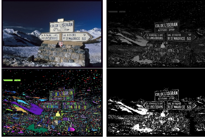
Figure 2. CCs extraction: From left to right and up to down: Original Image I , R_\theta(I) (Gamma Corrected \gamma = 3 ) and q_\theta(I) (randomized), detected CCs.
