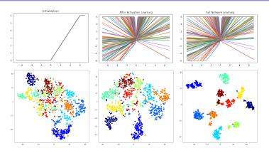
Left: Random Initialization with (14%) of performance on the test set, We use a simplified version of proposed activation  $\min(\max(\beta_0x + \alpha_0, \beta_1x + \alpha_1, \alpha_2), \alpha_3)$ , with initialization  $\max(\min(\text{ReLU}(x), 6), -6)$  Center: Training only activations (92.38%), Right: Training Full Network (98,58%). Second Row: t-SNE visualization of last layer is the 10-classes MNIST prediction for a CNN
